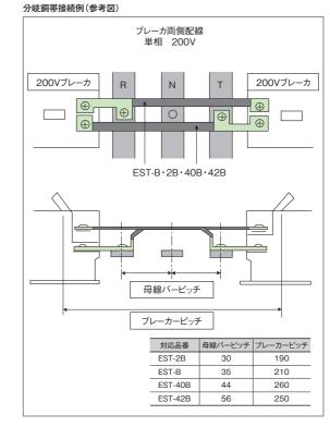
CONNECTING BARS FOR BRANCH CIRCUIT
