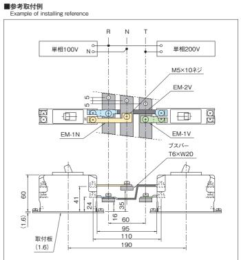
CONNECTING BARS FOR BRANCH CIRCUIT
