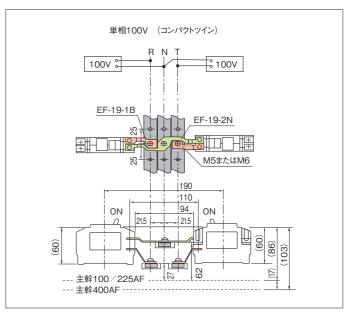
CONNECTING BARS FOR BRANCH CIRCUIT
