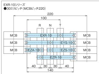
CONNECTING BARS FOR BRANCH CIRCUIT
