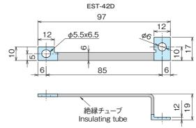
CONNECTING BARS FOR BRANCH CIRCUIT
