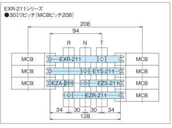
CONNECTING BARS FOR BRANCH CIRCUIT
