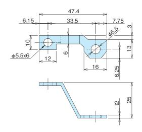
CONNECTING BARS FOR BRANCH CIRCUIT
