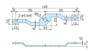
CONNECTING BARS FOR BRANCH CIRCUIT
